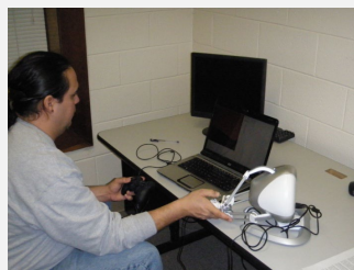
Technician performing engine inspection with VR borescope using haptic device
