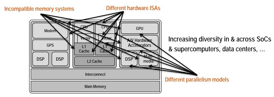
Need common interface (abstractions): HW-independent SW development, "object code" portability Data movement critical: Memory structures, communication, consistency, synchronization Approximation: Application-driven solution quality trade off to increase efficiency
