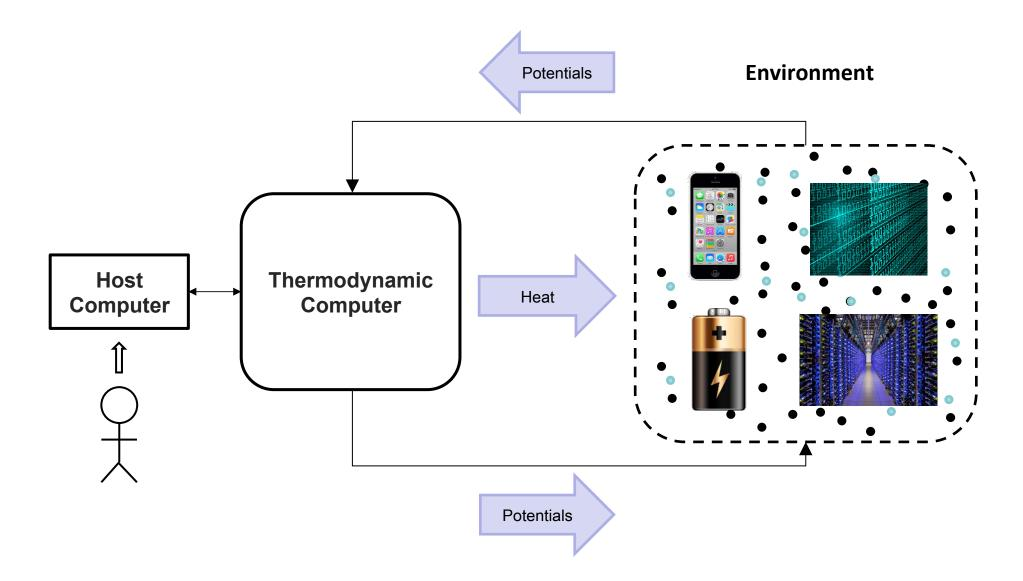
Thermodynamic Computers are open thermodynamic systems embedded in an environment of electrical and information potential.
