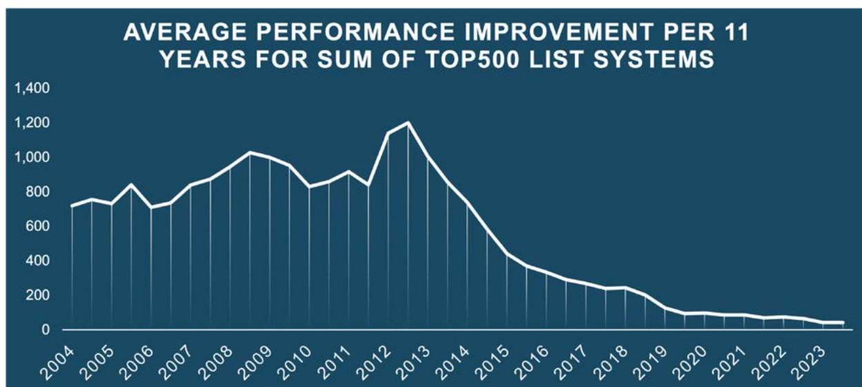
Figure 1: The performance growth rate of HPC systems (as measured by LINPACK) has slowed from its historical growth rate of 1000x every 11 years down to just 3x for the same time period in 2023. (figure from Shalf Supercomputing 2024 Top500 BoF)
